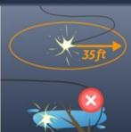
Downed power lines can energize the ground up to **35 feet away.** Even more in wet conditions.
